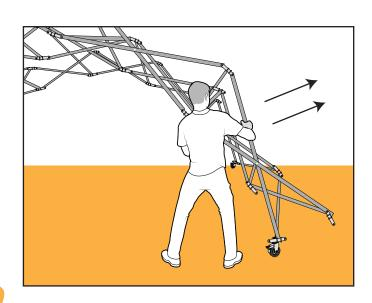
To fold the structure, you don't need power poles. Just lift and pull one side of the structure outward
